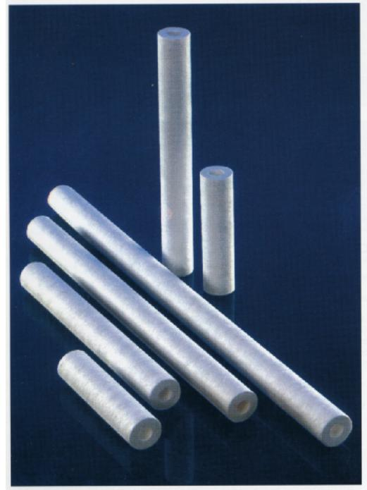
UltraBond® filter cartridges remove particulate more completely and over a longer period of time than any wound, molded spun type filter currently available. Filter-Mart's UltraBond® elements offer high performance due to a closely controlled melt blown manufacturing process. These cartridges consist of fibers that are very fine in diameter which build up the spun bonded layers of the media, thus providing the filter its depth. This process results in an
